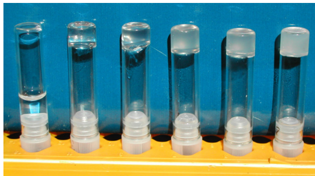
Figure 1. Gels formed by 3a in \text{CHCl}_3 at different concentrations at rt. From left: \text{CHCl}_3 only, 1.0, 1.5, 2.0, 2.5 and 3.0 wt%.
